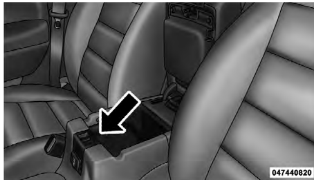
Center Console USB/AUX Connector Port
