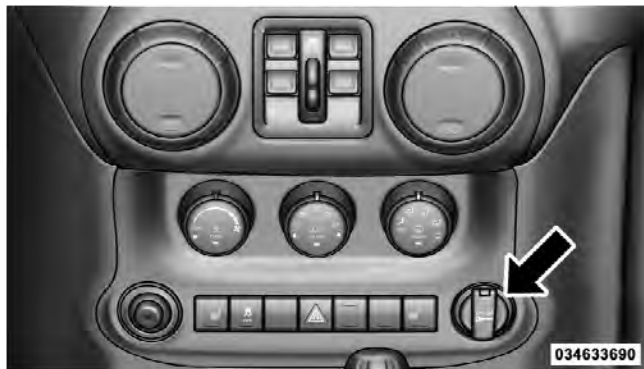
Front Power Outlet
