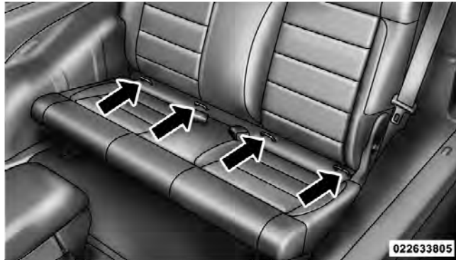
Latch Anchorages (Two-Door Models)
