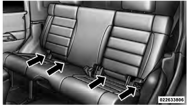
Latch Anchorages (Four-Door Models)
